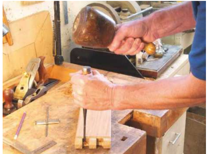
▲ Pic.12 Initial cleaning out of the hollows
